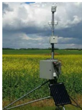
Above: Self-contained tripod deployed SW of Edmonton containing PurpleAir sensors, Aeroqual AQ, 2B OEM-106L and Vaisala WXT with solar/battery power.
