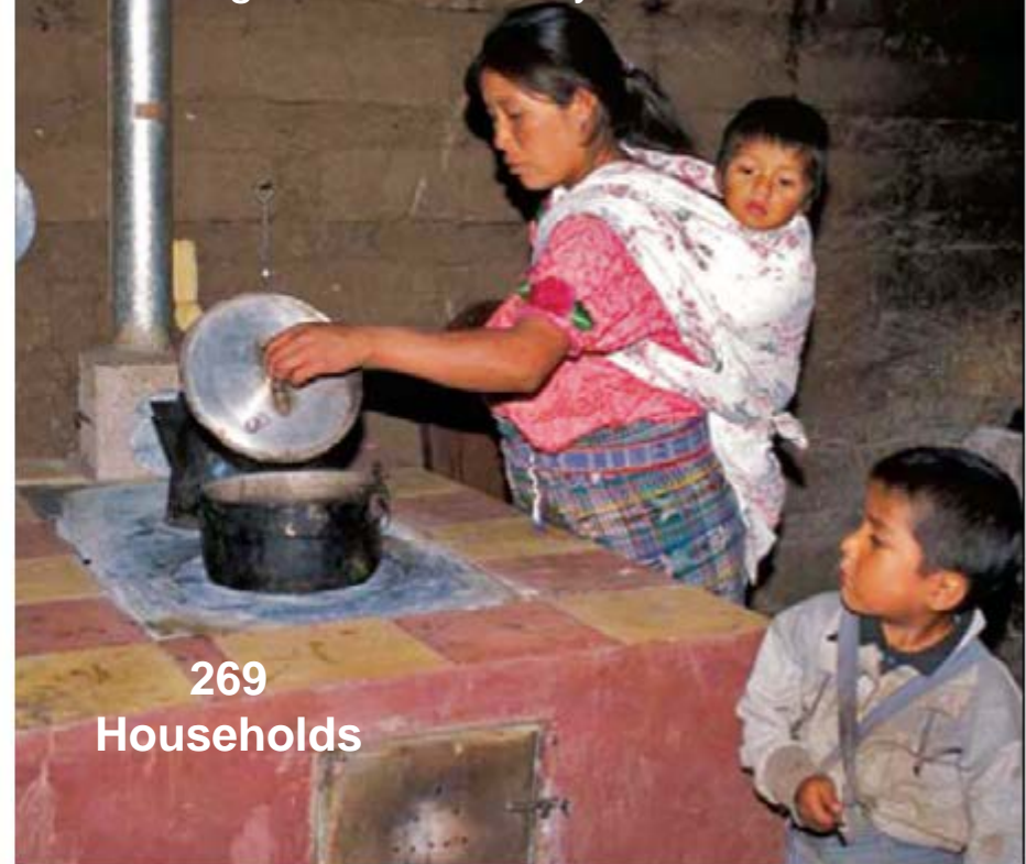
B Locally developed and constructed high-mass chimney woodstove
