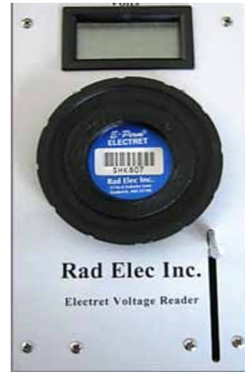
Image 2 – E-perm electret voltage reader
