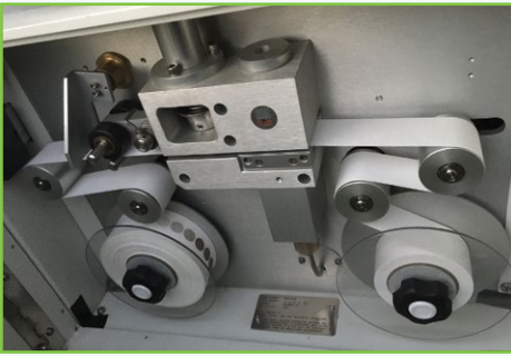
Figure 4. Filter tape in a Beta Attenuation Monitor (BAM). Each circular soiled mark on the left-hand tape reel represents one hour of PM_{2.5} collected in a community impacted by residential woodsmoke. The right-hand tape reel is unsoiled, and the beta attenuation measurements are made by the central unit.
