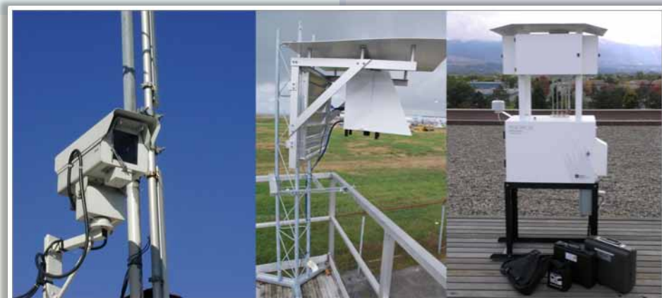
Fig. 15: Various instruments monitor visual air quality in Metro Vancouver and the Lower Fraser Valley. The camera on the left is programmed to take photos every 30 minutes for uploading to the Clear Air BC website. Nephelometers in the centre photo measure light scattering by particles and gases every hour. Scattering and light absorption measurements are combined to arrive at a near real-time measurement of visibility conditions. The speciated particulate matter (PM) sampler on the right collects fine particulate matter onto a filter over a 24-hr. period. Lab analysis helps determine which pollutants affect visibility degradation.
