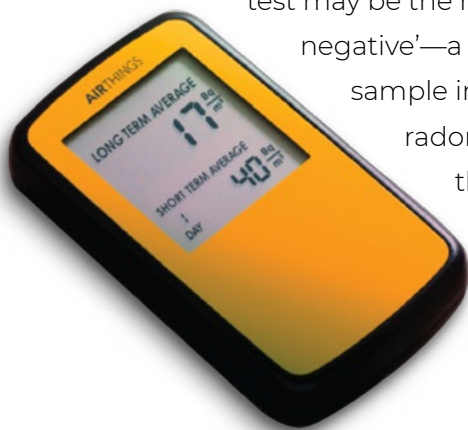
Fig. 4 A digital radon monitor
